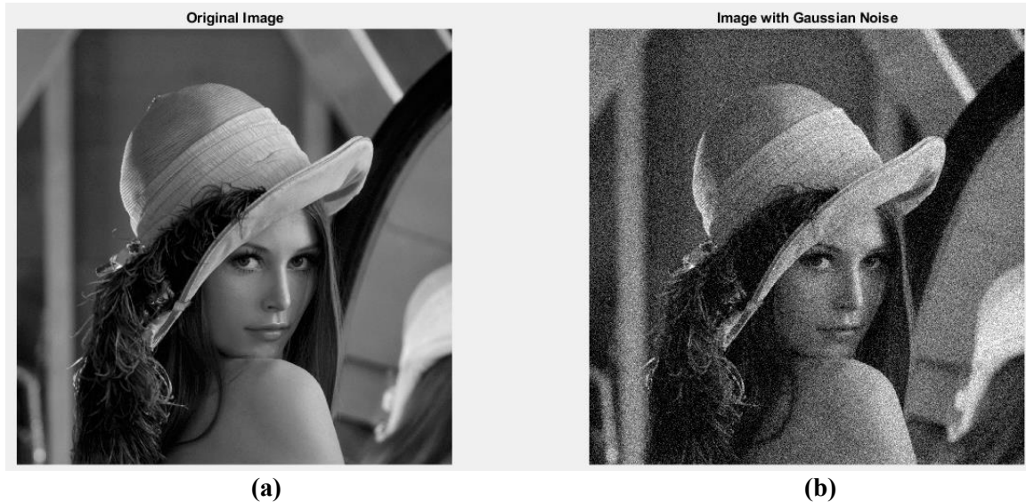
Figure 1. Grayscale image (a) Original Image (b) The Corrupted Image by Additive Gaussian Noise [9].
