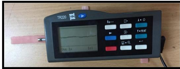
Figure 6: Surface roughness testing Profilometer.
